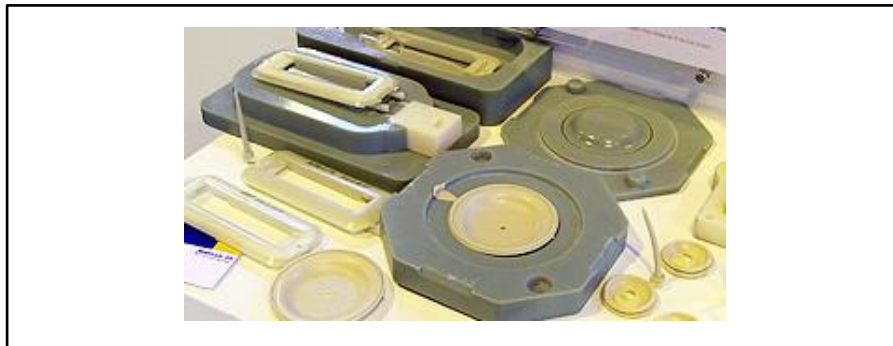
Figure 4.1.3.2. – Functional 3D printed injection mould.
